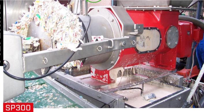
Since its introduction in 1998 the SP300 screw compression filter has proven its worth. This machine is ideally suited for the controlled dewatering and separation of various liquid waste and residue flows from industrial, organic and agricultural processes. With the help of an internal screw and filter, the liquid effluent is transported through the SP300. The resulting dewatered product which can in many cases be stacked, exits the machine via the delivery chamber.
